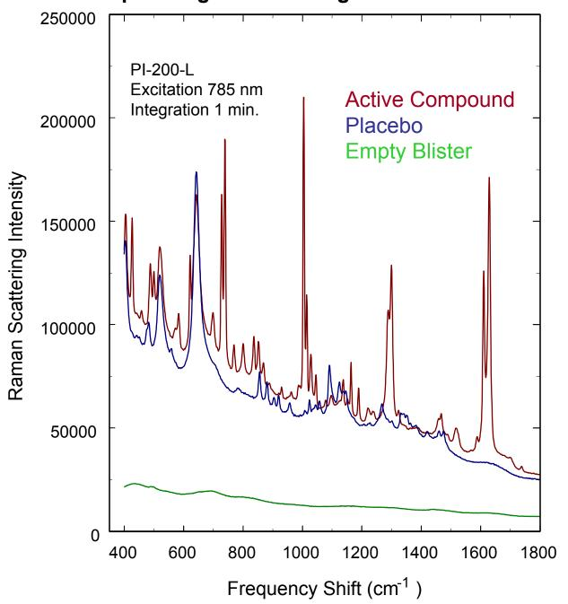
Spectral comparison between an active compound and a placebo where sample data acquisition was conducted through the blister pack. An empty blister pack spectrum is also displayed.
