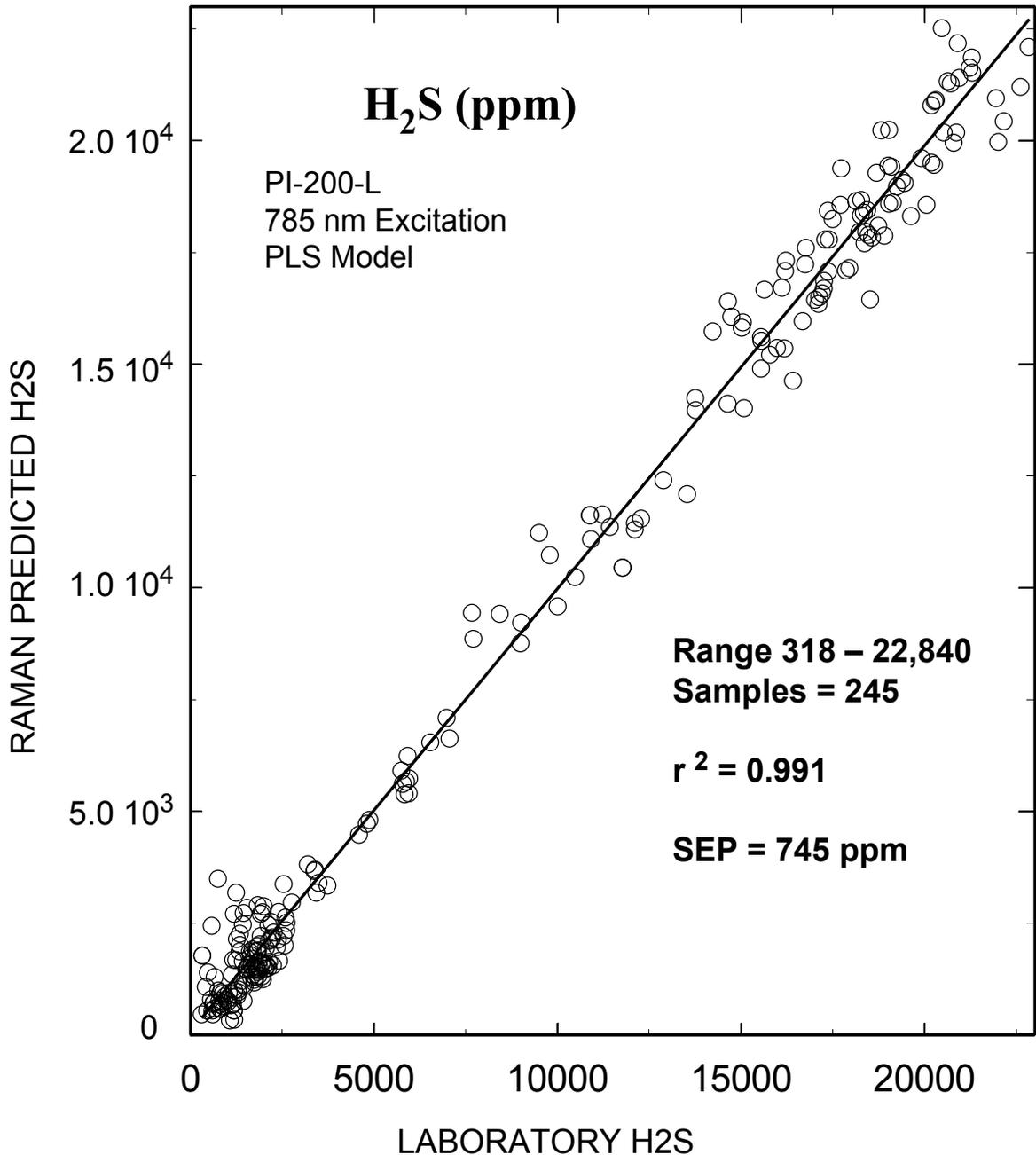
Typical on-line partial least squares (PLS) analysis of the H<sub>2</sub>S (ppm) concentrations. The plot shows Raman predicted values vs. the measured laboratory values. The standard error of prediction for the PLS model with outliers removed was 745.
