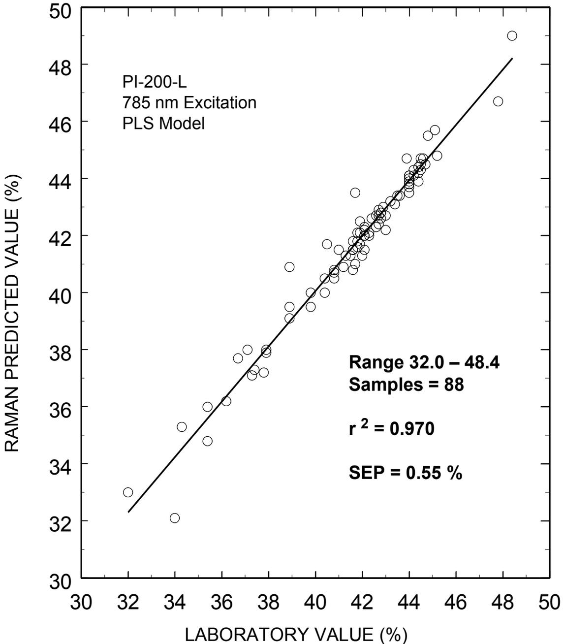
Typical on-line partial least squares (PLS) analysis of the MDEA concentrations. The plot shows Raman predicted values vs. the measured laboratory values. The standard error of prediction for the PLS model with outliers removed was 0.55 %.
