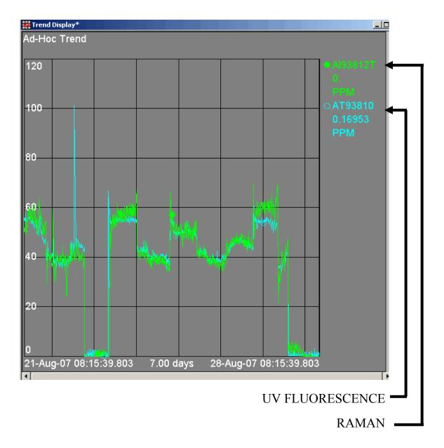
On-line Raman vs. On-line (UV Fluorescence) Ad-Hoc trend of sulfur measurements.
